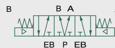
double air pilot 3 Position 4-Way (5/3), open to 4 (A) and 2 (B) in center
